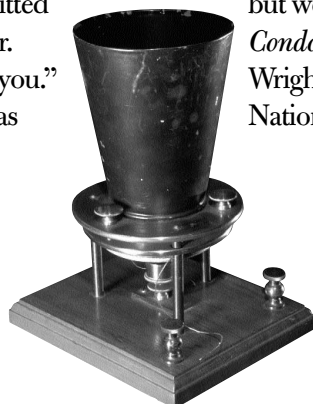
Bell’s liquid (variable-resistance) telephone transmitter
